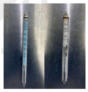
Note: (Left) Images depict the  $O_3$  (blue) and  $H_2O_2$  (white) readings prior to testing. (Right) Images depict the  $O_3$  (blue) and  $H_2O_2$  (white) readings immediately prior to carrier harvesting at the end of the contact time.
